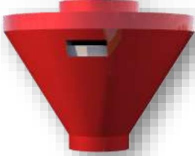
C'EST UN EQUIPEMENT QUI TRANSFERE LE CIMENT NECESSAIRE POUR LE MELANGE DU SILO AU MALAXEUR. L'EQUIPEMENT A UNE CAPACITE DE MESURE DE 50kg ET LA DECHARGE EST EFFECTUEE PAR LES VALVES PNEUMATIQUE SE TROUVANT AU DESSOUS DU MALAXEUR. LE CONTROL DE NIVEAU EST FAITE PAR L'OPERATEUR. LE PANNEAU ELECTRIQUE CONTIENT UN BOUTTON STOP-START. LE TRANSFERT DU CIMENT AU MALAXEUR EST FAIT A AIDE DES VALVES PNEUMATIQUES. LA DECHARGE PAR L'OPERATEUR EST FAIT VIA UNE MANETTE DE CONTROL.
