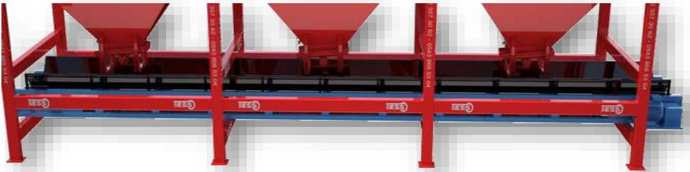
LA BANDE QUI TRANSFERT LES AGREGAT SE TROUVE JUSTE EN DESSOUS DU TREMIE. LE CHASSIS EST FAIT AVEC LES NORMES ISO 9001 ET EN RESPECTANT AUSSI TOUTES LES NORMES DIN DE 40 x 80 x 3 mm UN ÉPAISSEUR DU TOLE 3 mm. LES ROULEAUX SONT PLACES A CHAQUE 90 cm POUR EMPECHER LA FUITE DES PRODUITS. LA BANDE EST FAIT A 8 mm DE CORDON. LES ROULEAUX 3"( Ø 89 mm ) SONT PRODUITS DE FAÇONS STANDARD. ELLE A POUR PUISSANCE 2.2 kw. LA CONDUCTION EST TRANSMISE VIA LA POUILIE.
