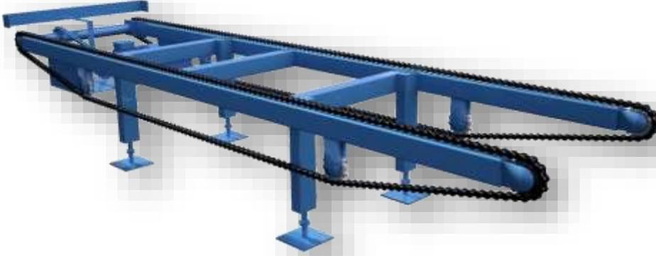
C'EST UN ÉQUIPEMENT ROBOTIQUE SUR LEQUEL LES PALETTES TRANSPORTANTS LES PRODUITS SONT RECUPERES ENVOYES VERS L'EMPILEUR DES PALETTES. ILS SONT CONDUITS PAR DES MOTEURS REDUCTEUR GRACES A DES DENTS ENCHAÎNEES. LE BOUTON (SWITCH) DEMONTRE L'ALLUMAGE ET L'ARRET DU FONCTIONNEMENT. LA CAPACITÉ DU MOTEUR EST 2.2KWDİR
