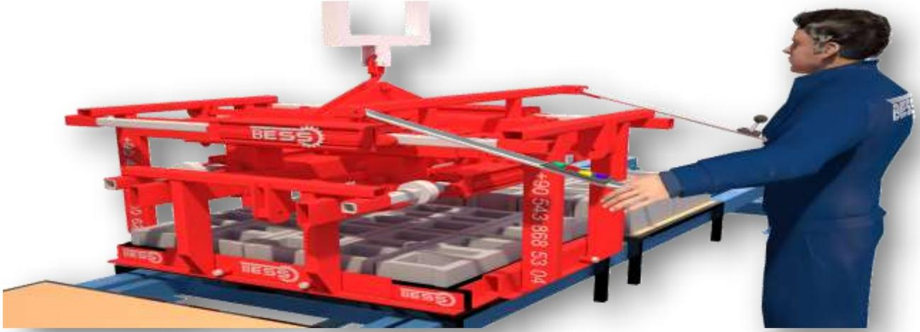
C'EST UN SYSTÈME PNEUMATIQUE EFFECTUER PAR LE MOUVEMENT DE LA PRISE EN CHARGE DES PRODUITS D EMPÏLAGE DU PALETTES D EXPEDITION, AU PRODUITS SÈCHES VENANT DU ROBOT DEPÏLEUR. LE MOTEUR EN MARCHÉ ET LE CROCHET MOUVANT DE GAUCHE VERS LA DROÏTE ET DU HAUT VERS LE BAS PERMET DE FAIRE RAPIDEMENT LE COLLECTE DES PRODUITS .LA PUÏSSANCE DU MOTEUR EST DE 0,2kw.
