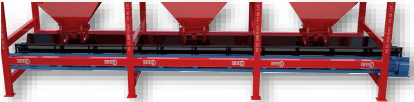
LA BANDE QUI TRANSFERT LES AGREGAT SE TROUVE JUSTE EN DESSOUS DU TREMIE. LE CHASSIS EST FAIT AVEC LES NORMES ISO 9001 ET EN RESPECTANT AUSSI TOUTES LES NORMES DIN DE 40 x 80 x 3 mm UN EPAISSEUR DU TOLE 3 mm. LES ROULEAUX SONT PLACES A CHAQUE 90 cm POUR EMPECHER LA FUIE DES PRODUITS. LA BANDE EST FAIT A 8 mm DE CORDON. LES ROULEAUX 3"( Ø 89 mm ) SONT PRODUITS DE FAÇONS STANDARD. ELLE A POUR PUISSANCE 2.2 kw. LA CONDUCTION EST TRANSMISE VIA LA POUILIE.
